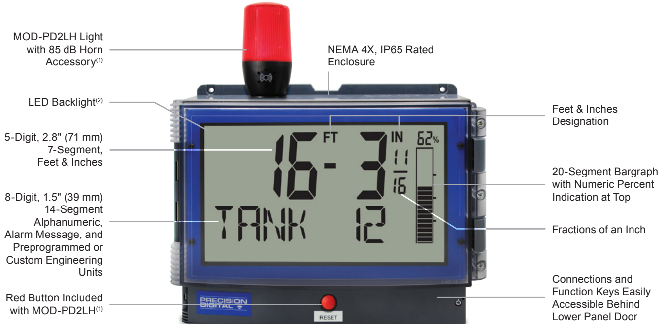
14-Segment Characters on Bottom Display Provide Clearer Readings of Units or Tags
