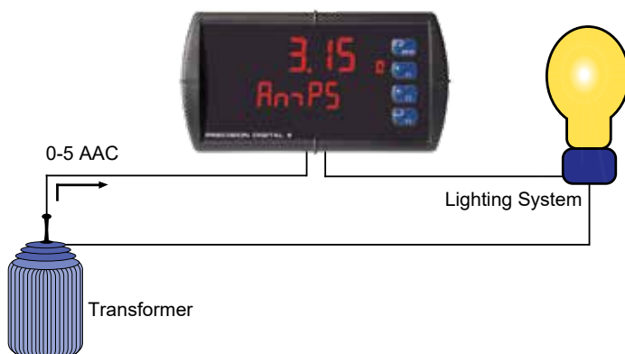
Current Input Application Example
