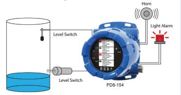
The ProtEX-MAX Annunciator is ideal for tank level switch monitoring.
