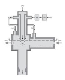
As a rule, measurements of dust content are required to state the concentration in mg/m3 or mg/dscm. But the intensity of the scattered light produced by a given dust particle depends greatly on particle characteristics such as size, shape, colour, relative density, etc.
